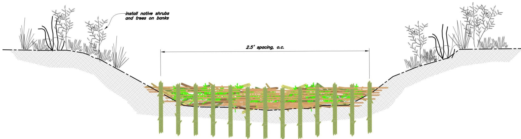
TYPICAL SECTION VIEW OF BEAVER DAM
