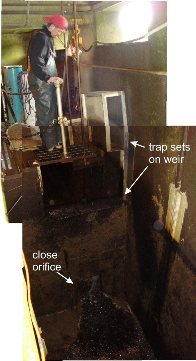
Figure 3. Lamprey trap sets on the top of a weir wall on Leg 2, prior to fish entering Pool 48, Sullivan Plant, Willamette Falls, Willamette River, OR.
