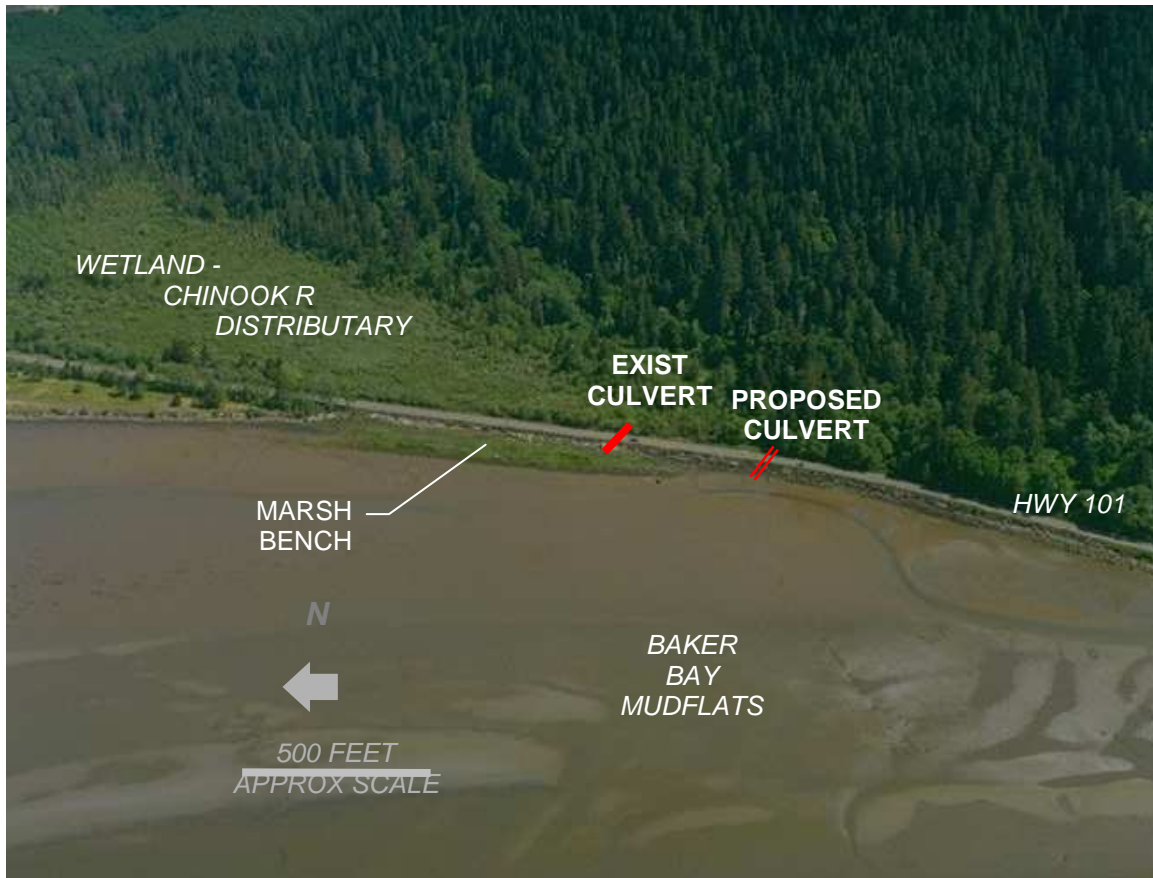
Figure 8 Alternative Culvert Locations.
