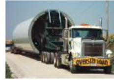
Step 4: Tower Sections are Delivered
