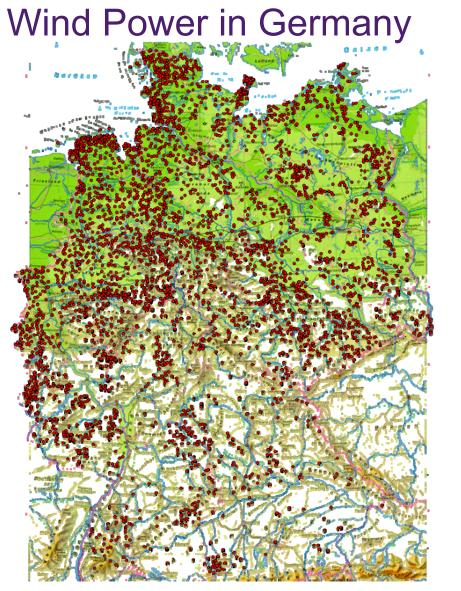
location of installed wind turbines
