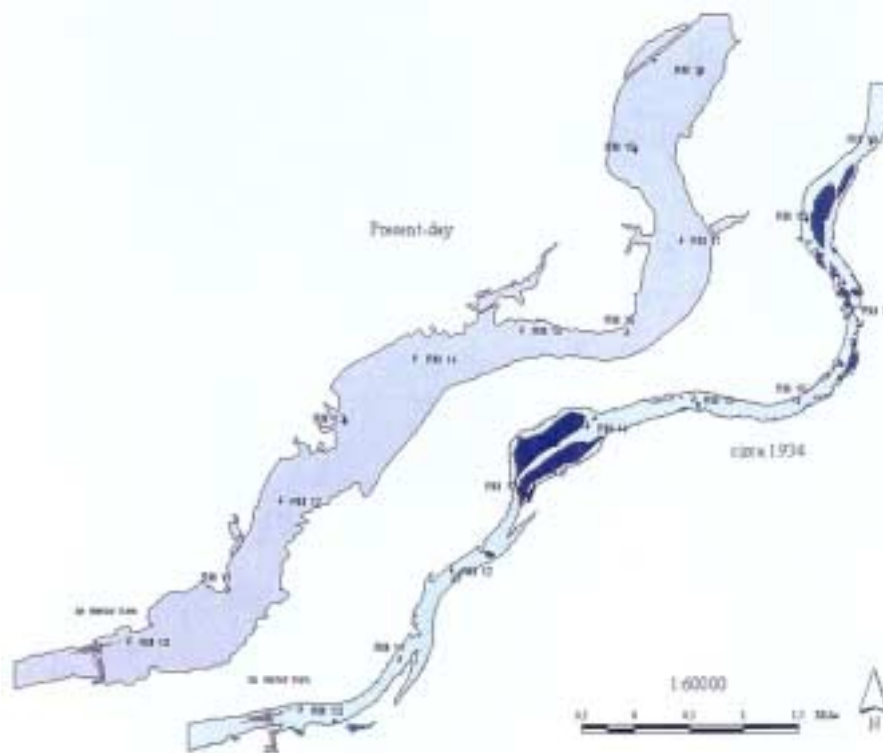
Figure 12.4. Lower Snake River planform channel morphology upstream of Ice Harbor Dam under present reservoir conditions (Lake Sacajawea) and pre-dam riverine conditions (1943) (Batelle's Pacific Northwest Division and the U.S. Geological Survey 2000).
